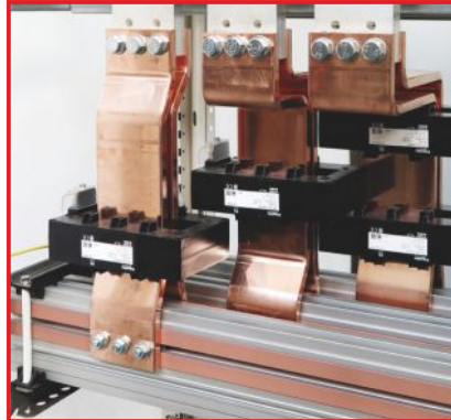
Bilateral connection of 2x80x10 mm busbars
